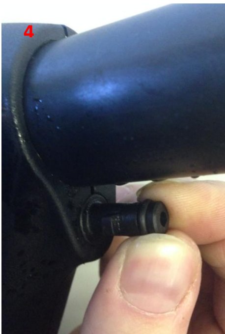
Check the o ring is positioned within the grooves on the pin
