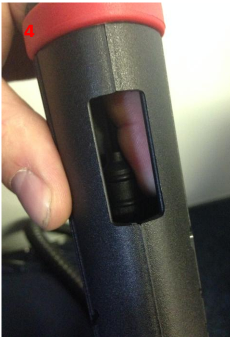
Check the o rings are positioned within the grooves on the pin
