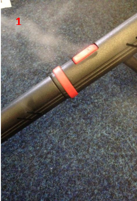
Steam leaking from the hose handle
