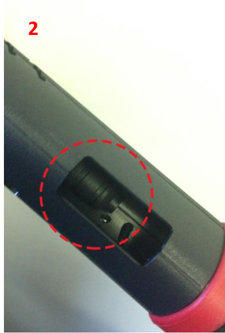
O rings maybe missing or damaged
