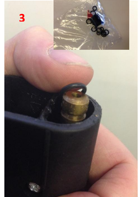
Replace the 2 x O rings on the steam pin
