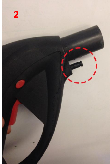
O ring maybe missing or damaged
