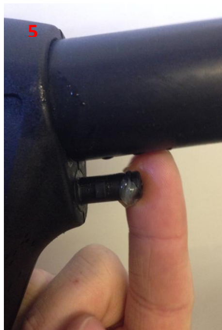
Grease the O rings on a regular basis to preserve the life and help with the removal of the accessories.
