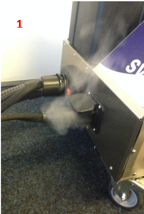
Steam leaking from the front of the machine
