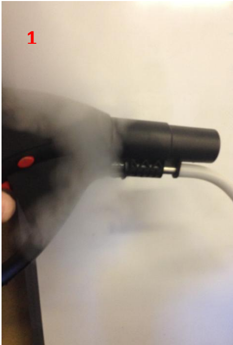
Steam leaking from the hose handle
