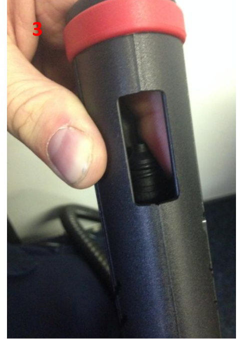
Replace the 2 x O rings on to the steam pin
