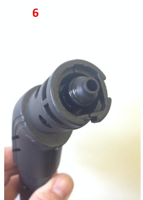
You can change and grease the o rings on this accessory (elbow) in the same way
