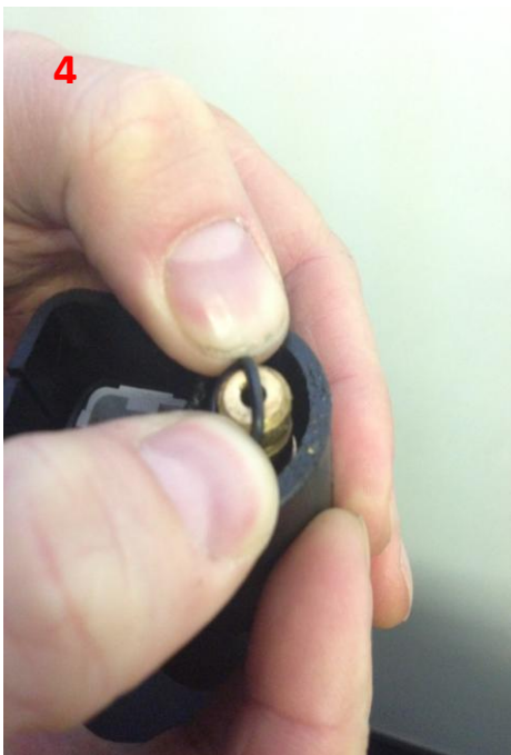
Roll the second O ring over the top of the first one for ease
