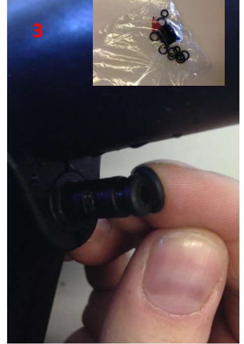
Replace the O ring on to the steam pin
