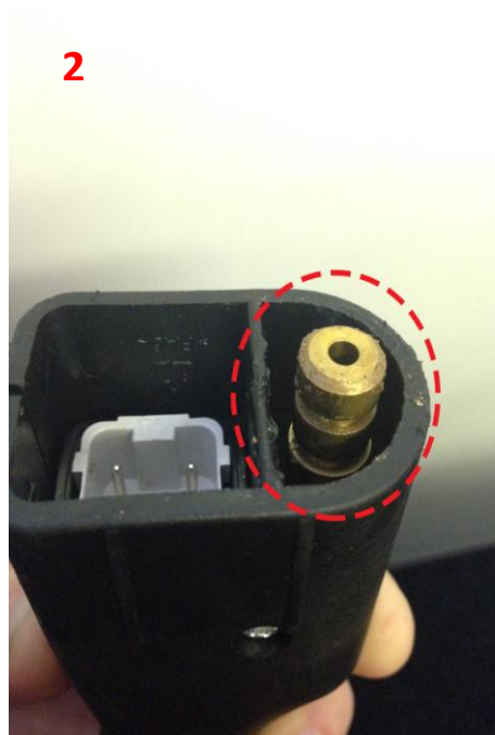
O rings maybe missing or damaged
