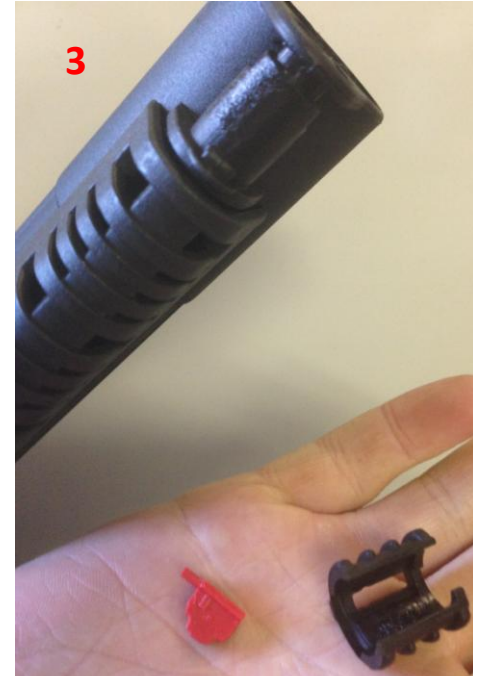
3 Discard Old and replace with new clips
