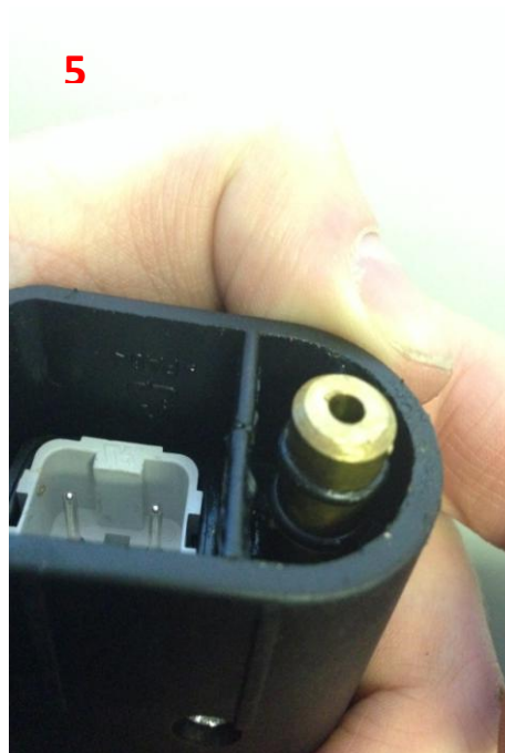
Check they are both positioned within the grooves of the pin
