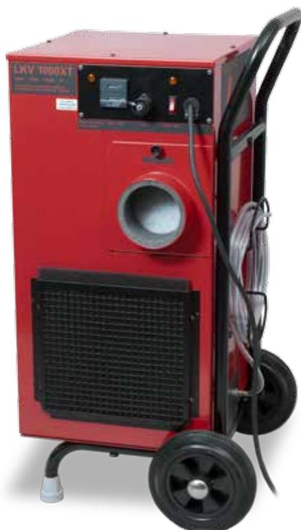
The machine automatically pumps out the condensation water, to a maximum pump height of 4 metres. It also dehumidifies at low temperatures and supplies the room with 3 kW of heat during operation, despite a low energy consumption of only 1.7 kW. CTR LKV 1000XT has a capacity of 20 l/day.
